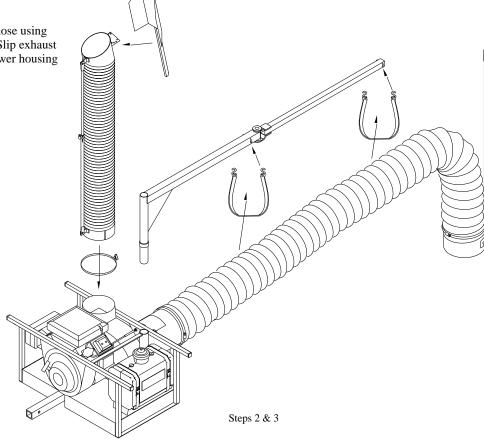
4.) Slip entire assembly into reese hitch and secure with 5/8" bent pin and hairpin clip. Loosen clamp on hose support on the metal exhaust hose and bend hose to the desired location and resecure clamp.
