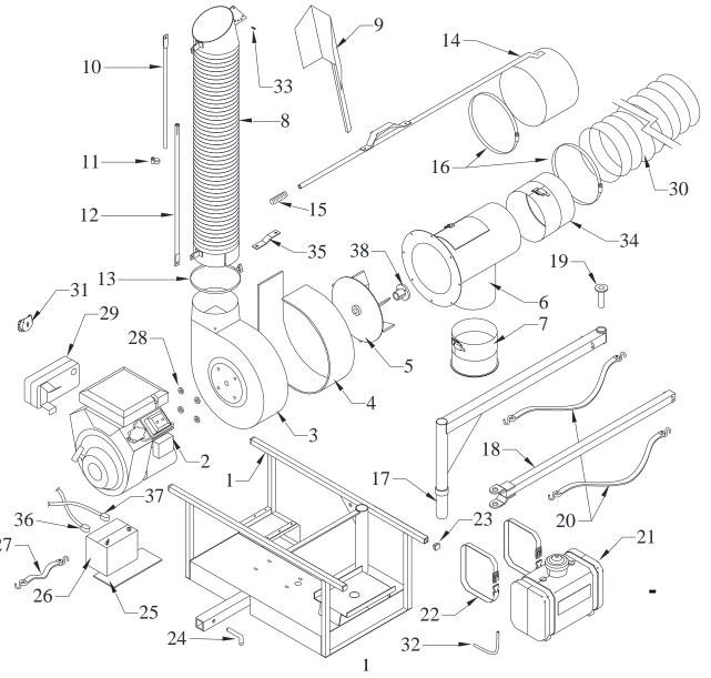
1.) Slip 10" hose clamp over hose and slip hose over inlet and secure. Repeat same procedure at opposite end of hose with the hand wand.
