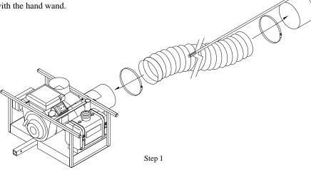
2.) Drop hose support arm into receiver on frame of vac. Connect support arm extension to support arm with the 1" diameter pin and attach 10" hose to hose support assembly with 31" tarp straps provide.
